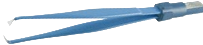
Bipolar multifunctional forceps, inside angled, length 130 mm, wide 3 mm
