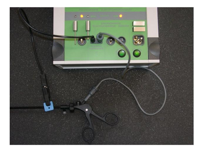
Connect the connection cable with clamp and the instrument cable to the "Insulation" sockets of the cable test unit.
